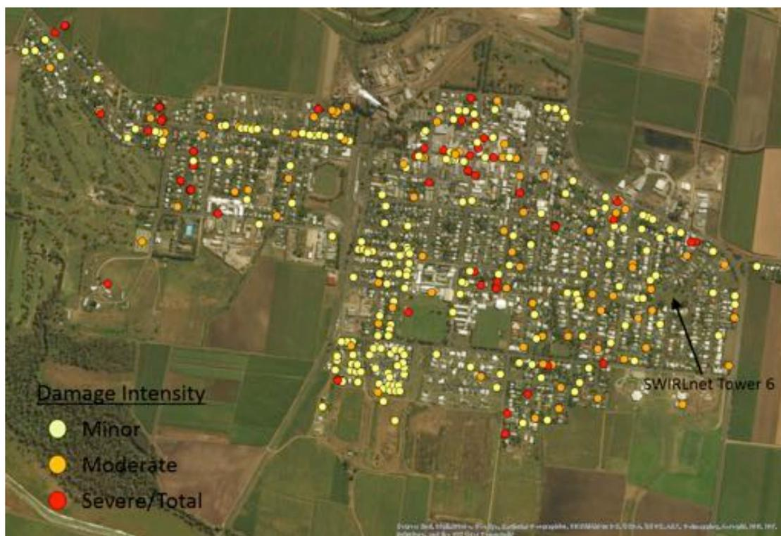
**Figure 3.2. RDA damage points in Proserpine from TC Debbie (undamaged buildings are not shown)**
