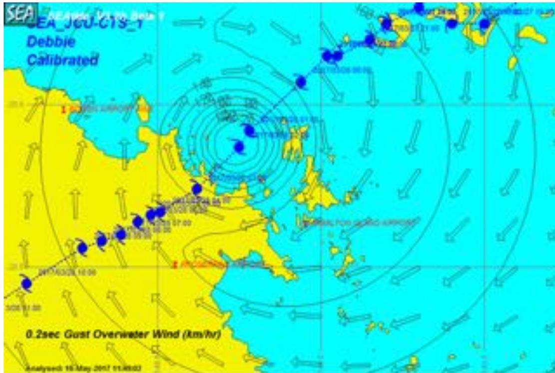
**Figure 2.7 3-second Holland model results of wind before landfall**
