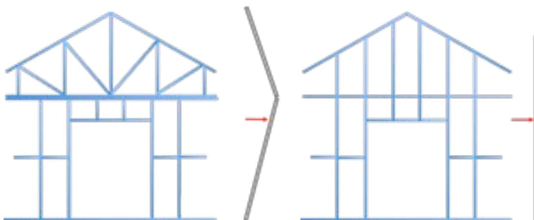
(a) Separate wall frame and truss
