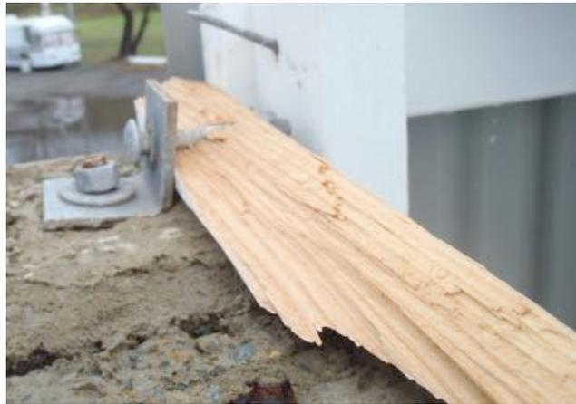
**Figure 7.21 Failure of roof beam in tension perpendicular to grain
