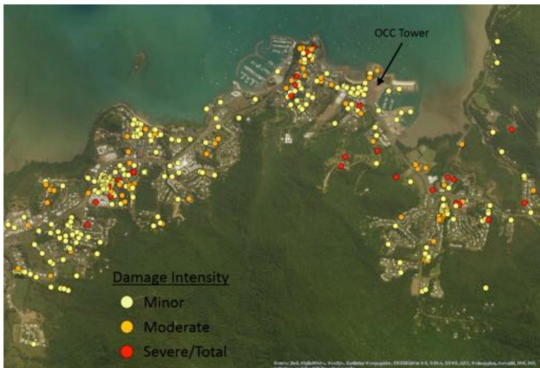
Figure 3.4 RDA damage points in Airlie/Cannonvale from TC Debbie (undamaged buildings are not shown)
