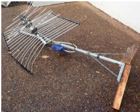
(a) Aerial lost due to inadequate roof fixing
