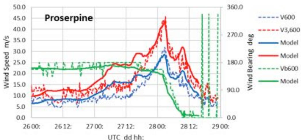
**Figure 2.8 3-second Holland model results and AWS data for Proserpine**
