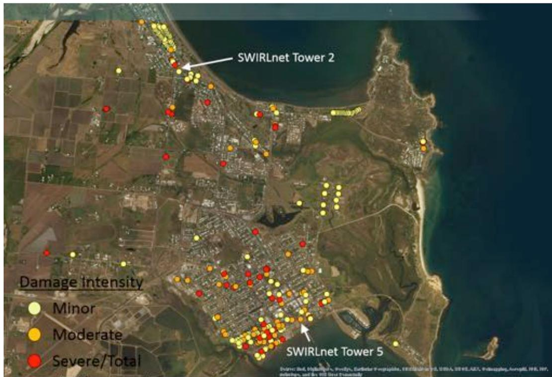
Figure 3.3 RDA damage points in Bowen from TC Debbie (undamaged buildings are not shown)
