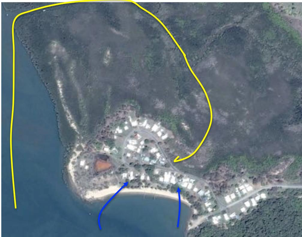
**Figure 6.4 Directions of storm tide inundation at Wilson Beach**
