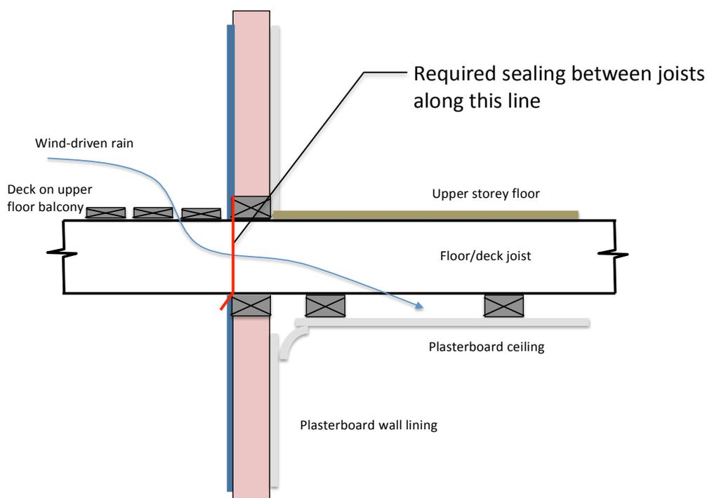
Figure 5.17 Diagram of seal required at junction of deck and external wall
