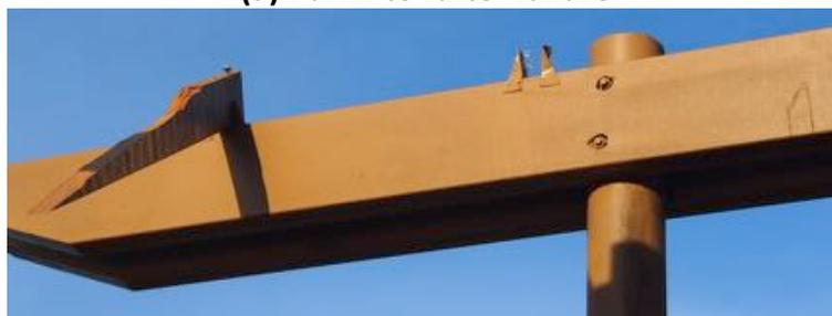
**(b) Tension perpendicular to grain in purlin**
