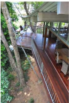
This design optimises the use of natural light and ventilation. With glass panel doors on both sides of this narrow house artificial lighting is minimised. Ceilings curving up to a central loft space promote a rising air flow. This is boosted by drawing cool air through gaps in the floor and ceiling fans so a natural cooling of the whole body is achieved.
