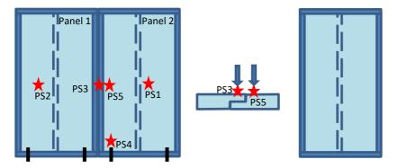
Figure 7.2 Locations of debris test impacts on wall panel systems
