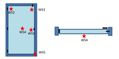
Figure 7.4 Locations of debris test impacts on window systems (casement shown)
