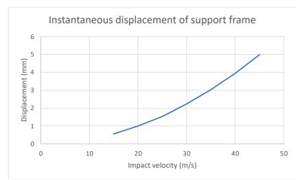
Figure 6.2 Relationship between displacement of the support frame and impact velocity
