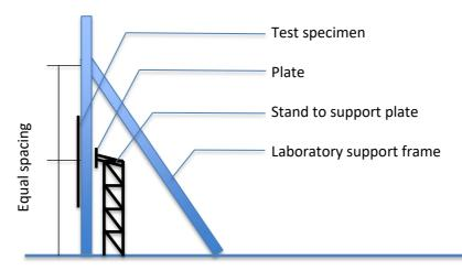
Figure 6.1 Configuration for the check for support frame displacement
