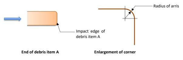
Figure 6.3 Arrises on the end of Debris item A
