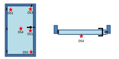
Figure 7.3 Locations of debris test impacts on door systems
