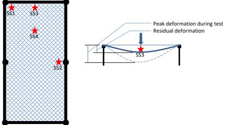
Figure 7. 5 Locations of debris test impacts on shutters and screens
