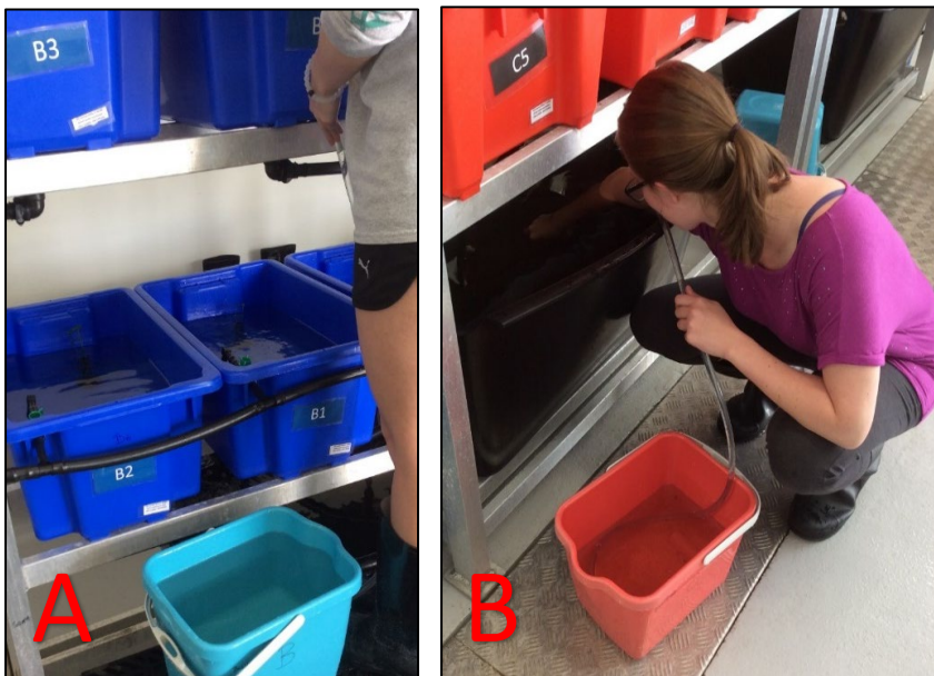
Figure 10. A) Use the system bucket to collect the water you have siphoned out. B) On certain days the sumps are siphoned. Use the system bucket to collect debris.
