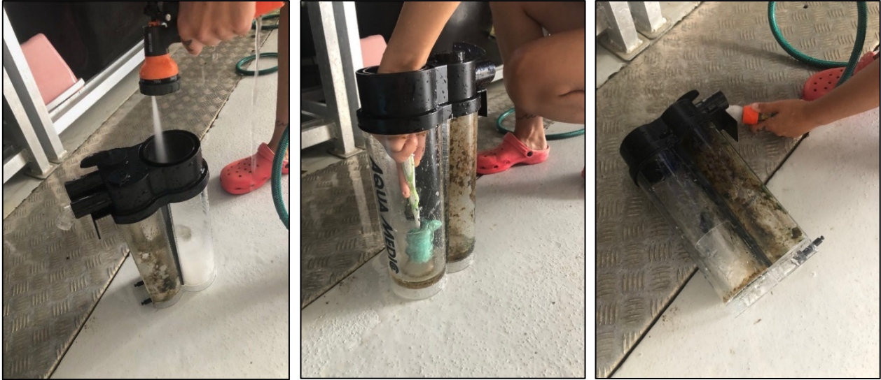
Figure 13. Use the hose and toothbrush with chux to clean hard to reach areas.
