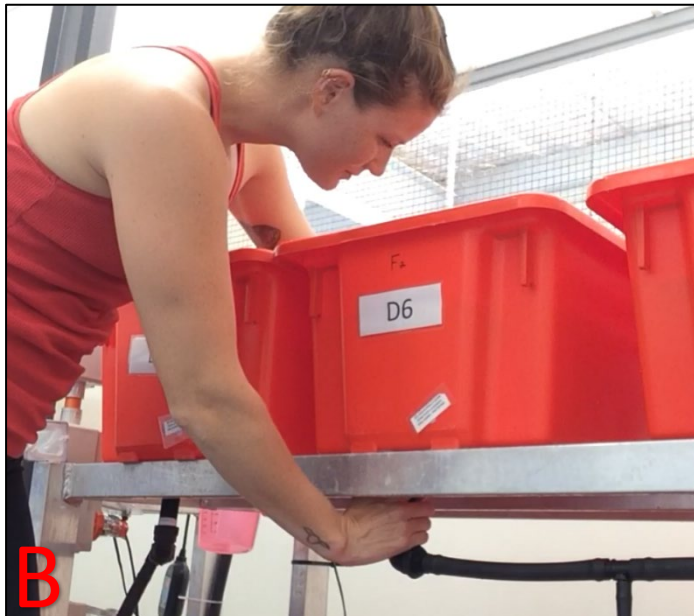
Figure 34. A) If the bolt comes loose, the tank may begin to leak. This is the part you need to hold when unscrewing the standpipe. B) Hold the bolt in place while unscrewing the standpipe during a water exchange.
