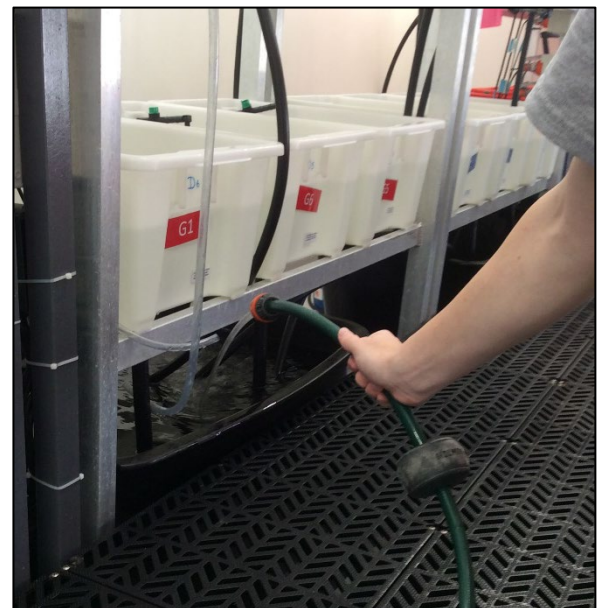
Figure 37. The hose nozzle should not touch the water within any system when adding water to the sump or to the tanks. This reduces any cross-contamination between systems.
