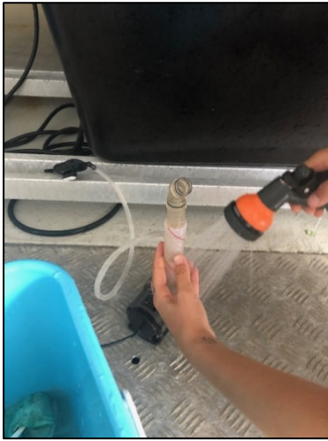
Figure 14. Gently rinse and wipe down pump system to remove organic waste buildup.
