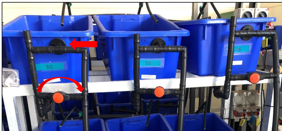
Figure 33. Newer systems have external standpipes that give us the flexibility to have water flow out of the tanks via the bottom or the side of the tank. To drain a tank that is using an outlet at the side of the tank (where red arrow is), turn the valve parallel to the poly pipe open to allow water to drain.
