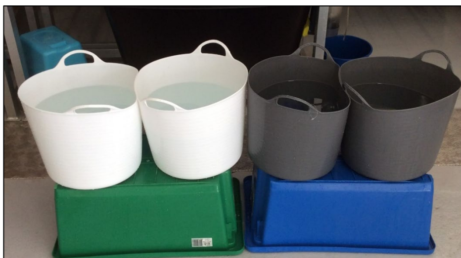
Figure 4. Set up the rinse bins to get ready to wash equipment according to proper protocol (refer to Rinsing Equipment ).
