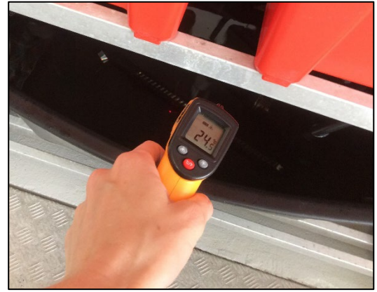
Figure 36. Use the heat gun to check the temperature in the sump or holding tank. Push the trigger and allow the reading to steady.
