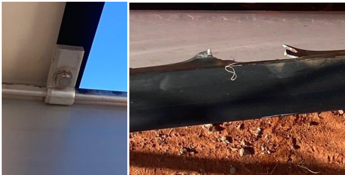
Figure 3-10 Detail of the chassis failure.
