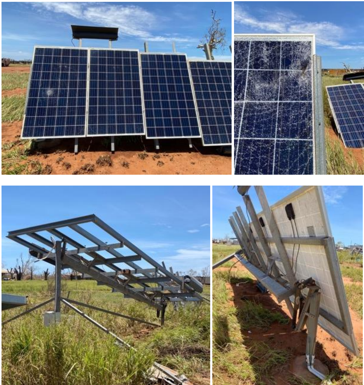
Figure 3-16 Damaged ground-mounted solar panels.
