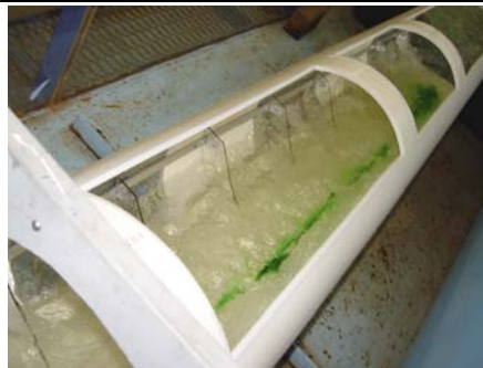
Two standard baffle height flow depth: Dye inserted on right showing unobstructed flow outside baffle field on right (18/08/06)
