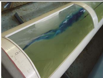
Three standard baffle height flow depth: Dye inserted on left showing unobstructed surface streamline swinging to centre (18/08/06)
