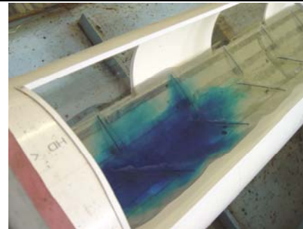
One standard baffle height flow depth: Dye inserted on right showing flow obstruction / shelter within baffle field on right (18/08/06)
