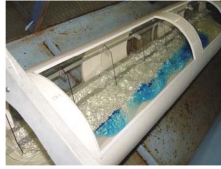
One standard baffle height flow depth: Dye inserted on right showing unobstructed flow outside baffle field on right (18/08/06)
