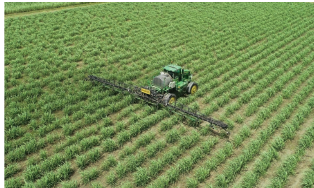
Figure 1: AutoWeed system in operating in a sugarcane field near Ayr, Queensland.
