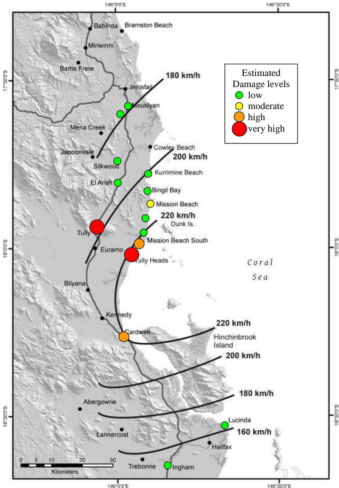
**Figure 3.1 Representation of early estimates of reported damage by EMQ overlaid on estimated wind field.**
