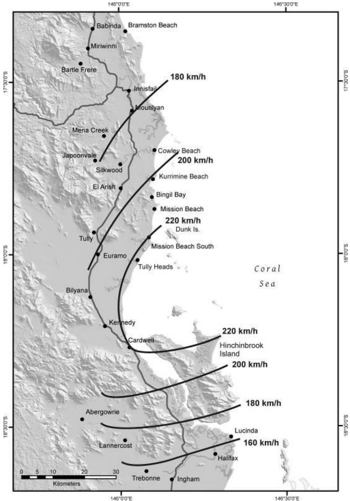
**Figure 2.7** Approximate contours of maximum 3-second gust at any time during the event (Topographic effects not included.)
