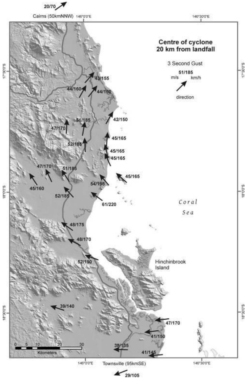
**Figures 2.4 Wind directions and gust speeds from Holland model – prior to landfall**
