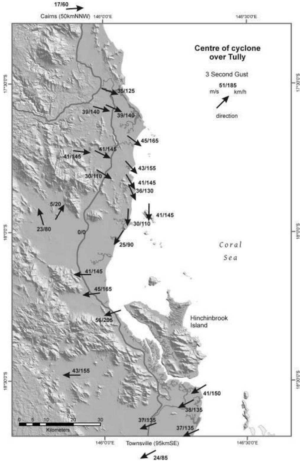
**Figures 2.6 Wind directions and gust speeds from Holland model – after landfall**
