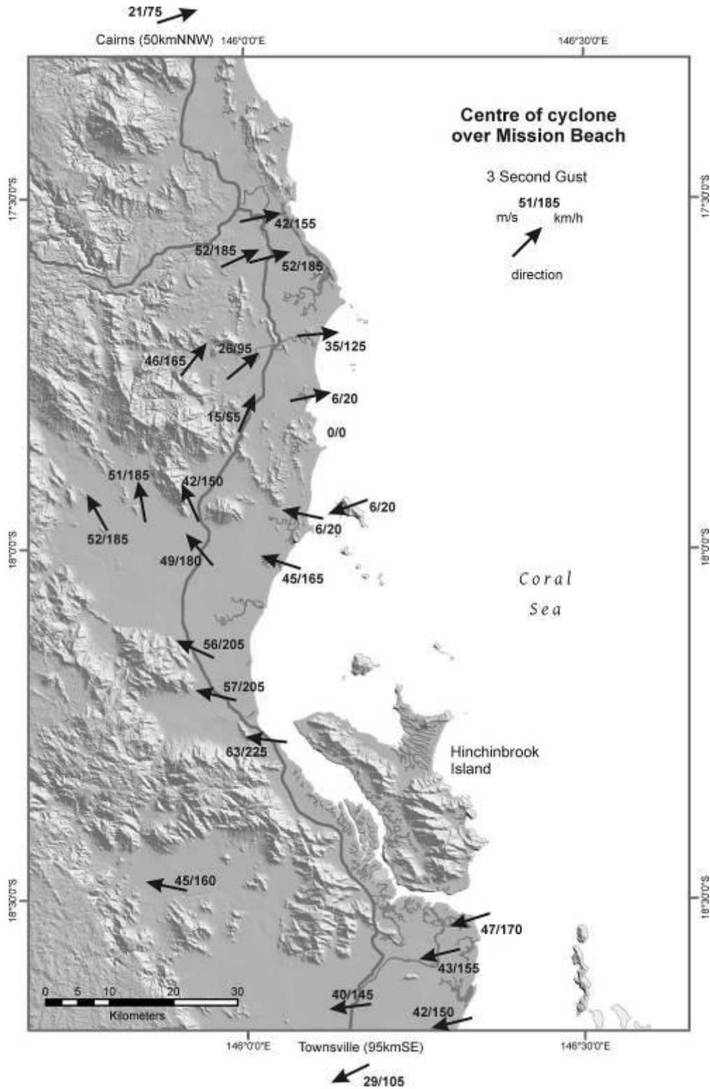
**Figures 2.5 Wind directions and gust speeds from Holland model – at landfall**
