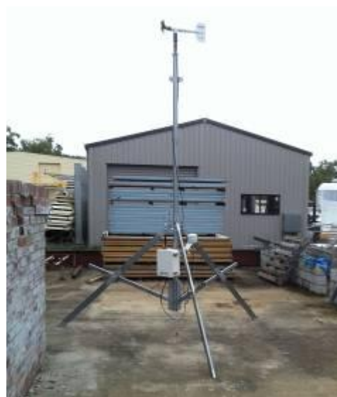
Prototype 3.5 m tripod on CTS house testing pad
