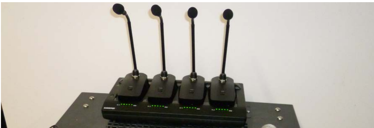
Image above showing wireless gooseneck microphones in charger on top of AV equipment rack.
