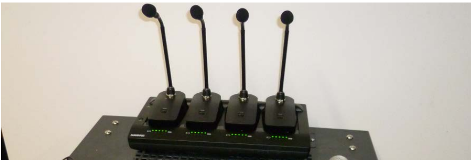
Image above showing wireless gooseneck microphones in charger on top of AV equipment rack.
