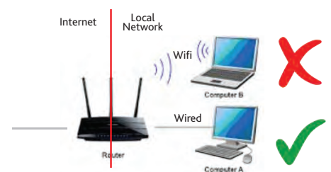
Wired connection to router = Good Wifi connection = Potential for trouble
