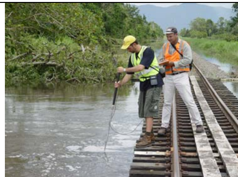
Field velocity measurements at rail bridge crossing of Murray River using current meter (24/03/06)
