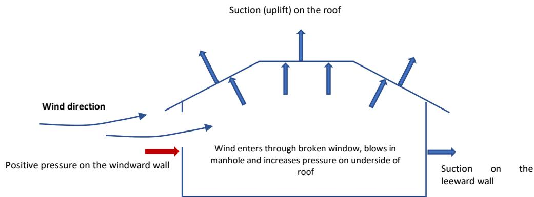
Figure 4-12 Net pressures across a roof
