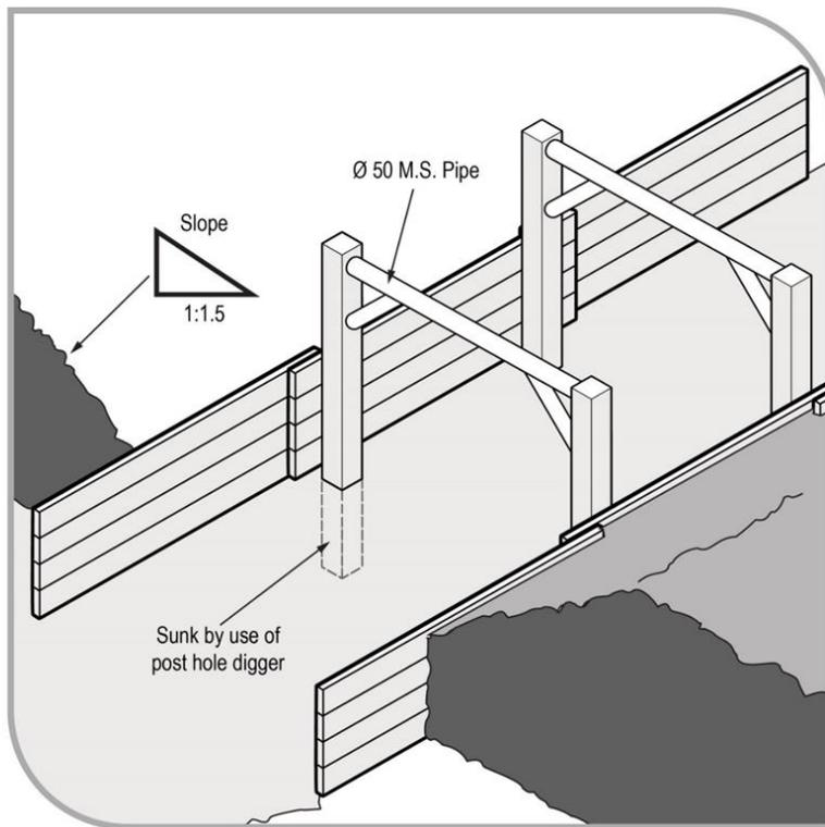
**Figure 17** Side lacing in sand trench
