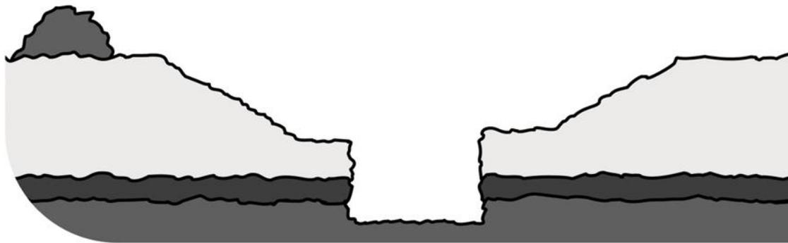
**Figure 11** Combination of benching and battering controls
