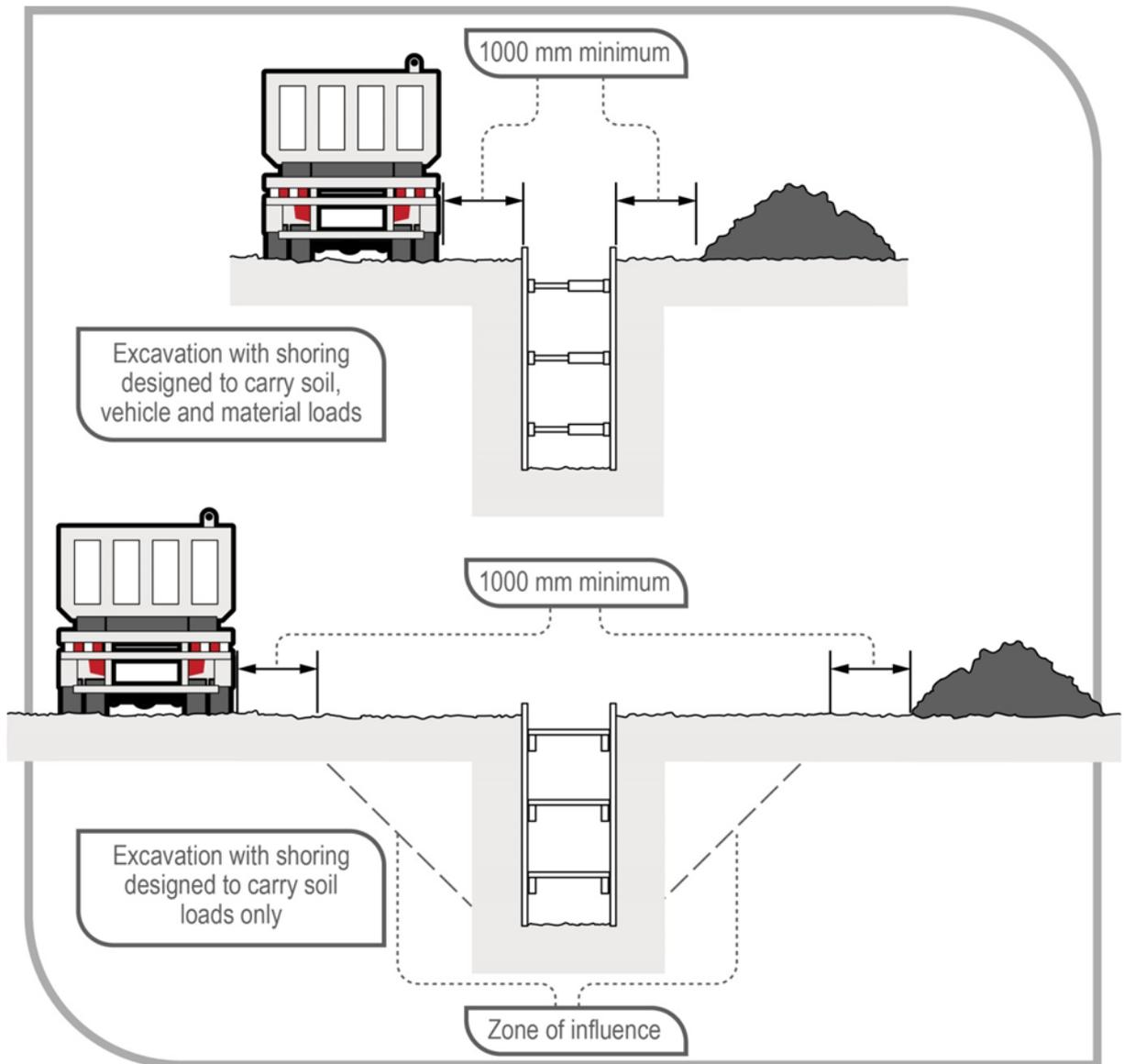
**Figure 2** Excavated material and loads near excavations
