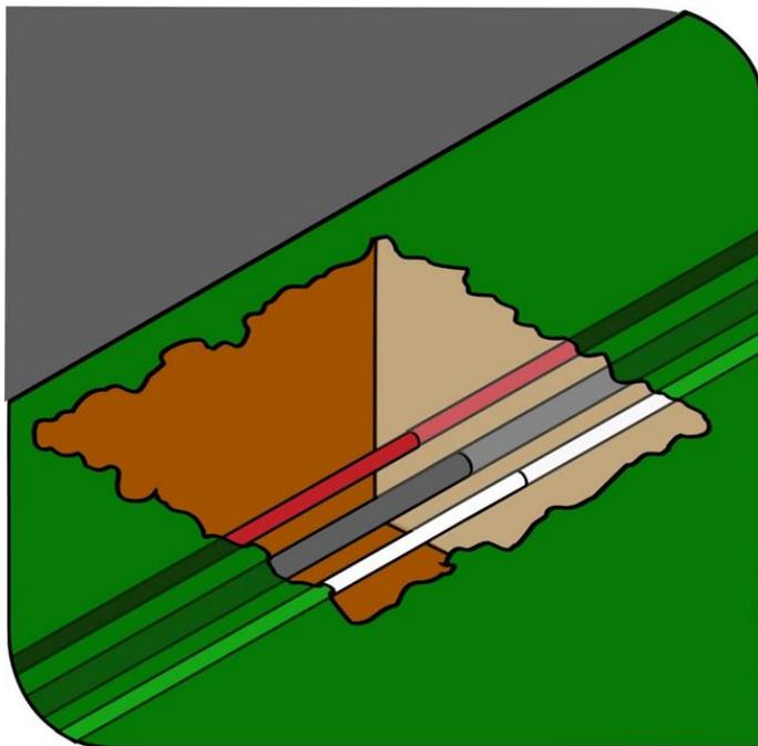
**Figure 1** Underground essential services exposed by potholing
