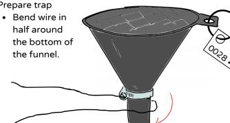
• Twist wire ends for ~5 cm, so the twisted part sticks out as far as the funnel's tab. The loose ends will be attached to the support.
