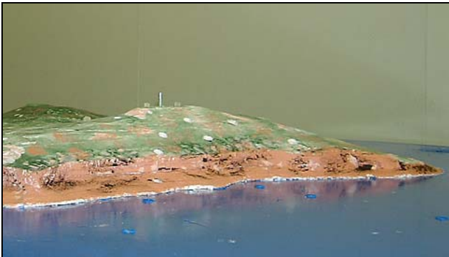
Wind tunnel model of the Cape Moreton AWS site
