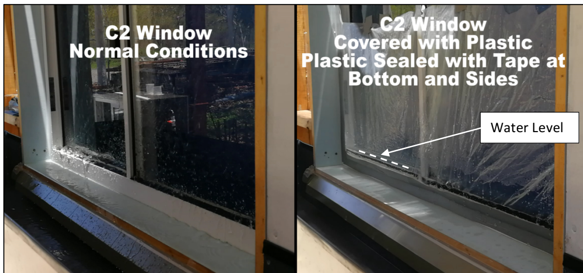
Figure 6 Side by side views of normal window and window with the Plastic sheet sill extension during a pressure peak
