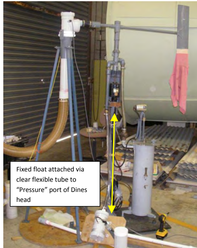
Figure 12. Dines head connected to fixed float volume
