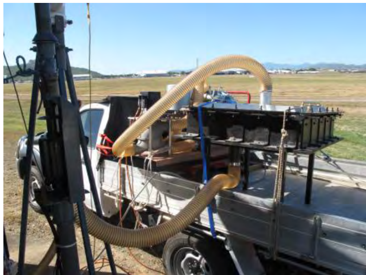
Figure 17. PLA (in utility) connected to volume chamber which is connected to high-speed Dines
