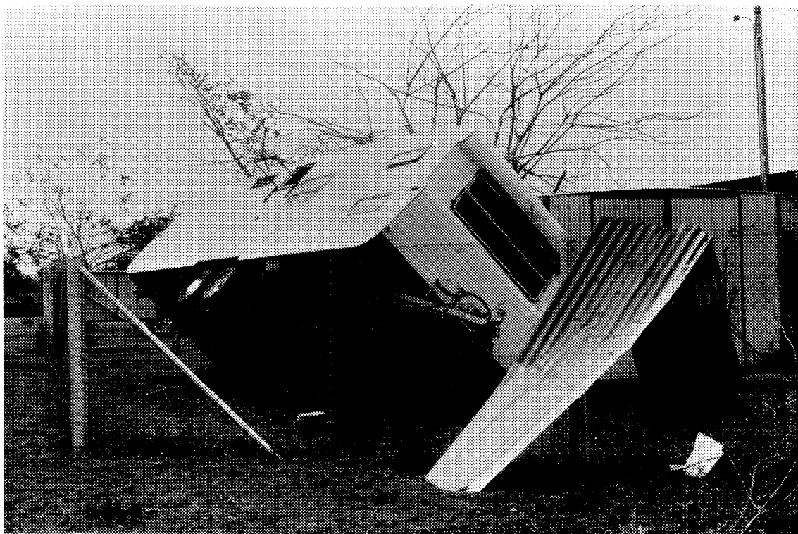
Figure 3 The force required to overturn this caravan was used to find a lower bound on the maximum wind gust.
