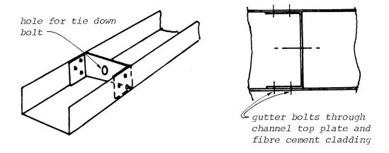
Figure 11. Redesigned bracket for window head.
