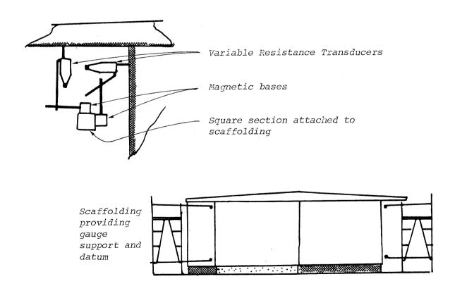
Figure 5. System for measuring deflections.
