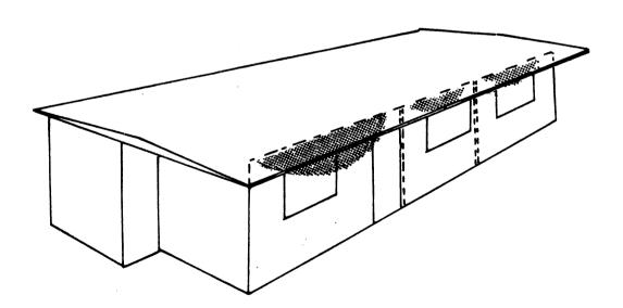
(c) Tributary area for roof resistance mechanism.
