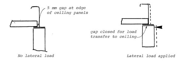
(b) Details of load transfer to ceiling panels.
