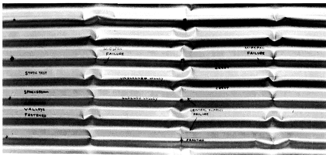
Figure 24. Ultimate Static Failure of Corrugated Roofing Fastened at Alternate Valleys
