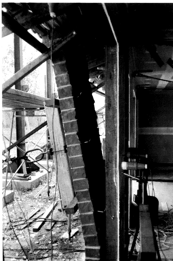
FIGURE 19 Bending Failure of Brickwork
