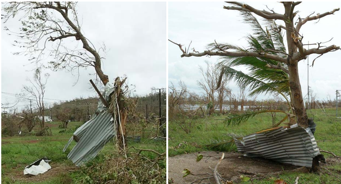
Figure 39: Examples of wind driven cladding (predominantly with battens attached)
