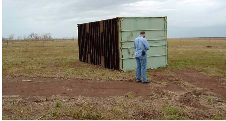
Figure 6: Empty container (lifted and overturned as no drag marks observed)
