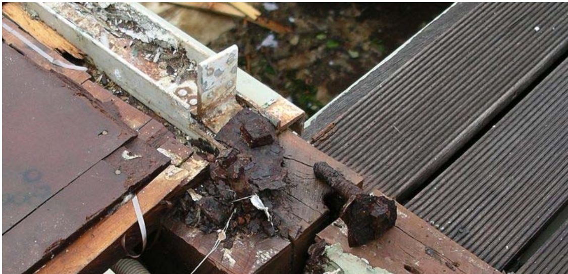
Figure 21: Aluminium inverted T bracket showing sheared rivets
