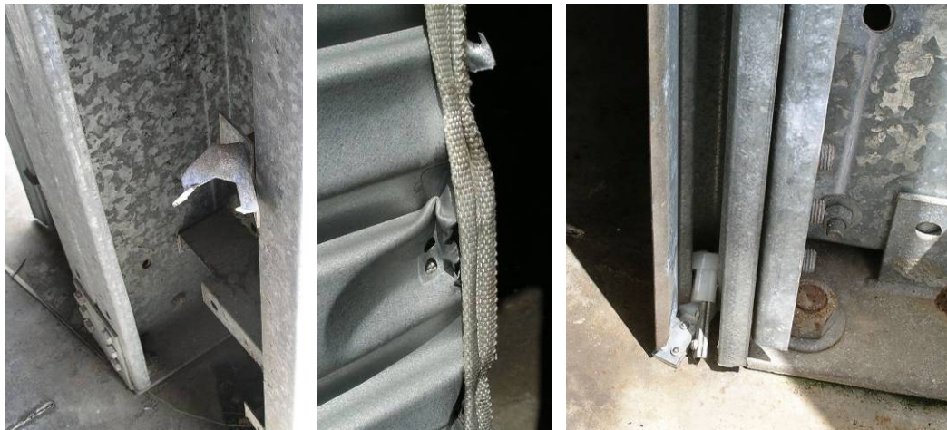
(a) Failed track bracket (b) Windlock torn from door (c) Wind lock in track
