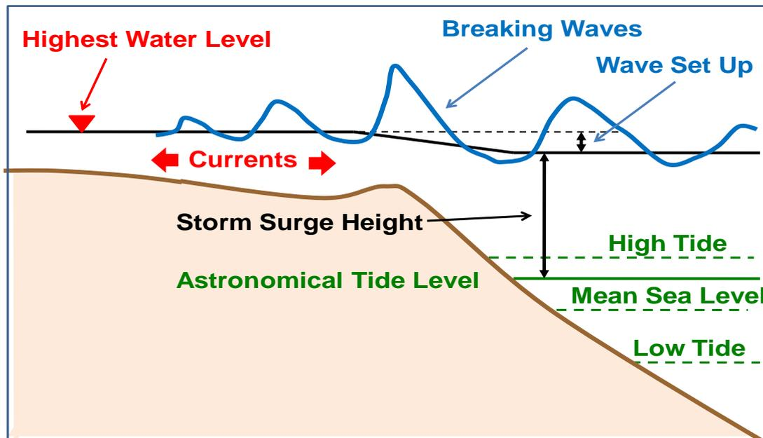
**Figure D.2 Schematic of Combination of Storm Surge, Tide and Waves at Coastline**
