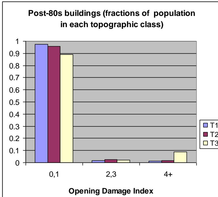
**Figure 3.5 Openings damage and topographic class for Post-80s buildings (Refer Table 3.1 for Damage Index values)**
