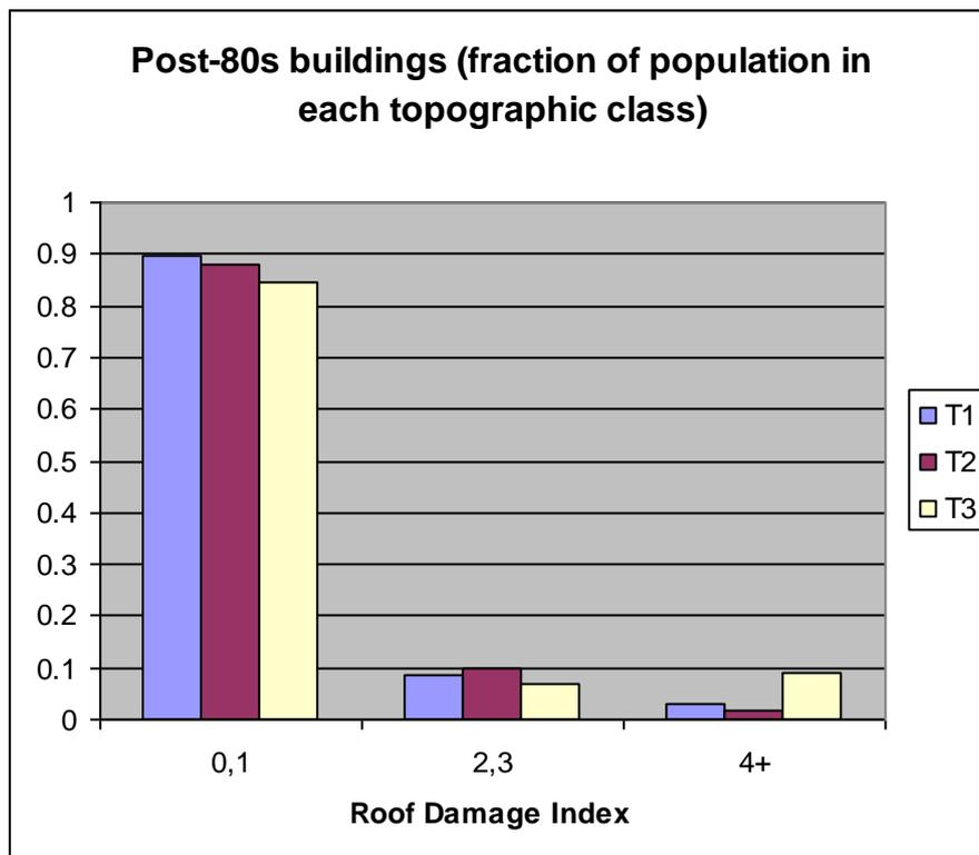
**Figure 3.4 Roof damage and topographic class for Post-80s houses (Refer Table 3.1 for Damage Index values)**
