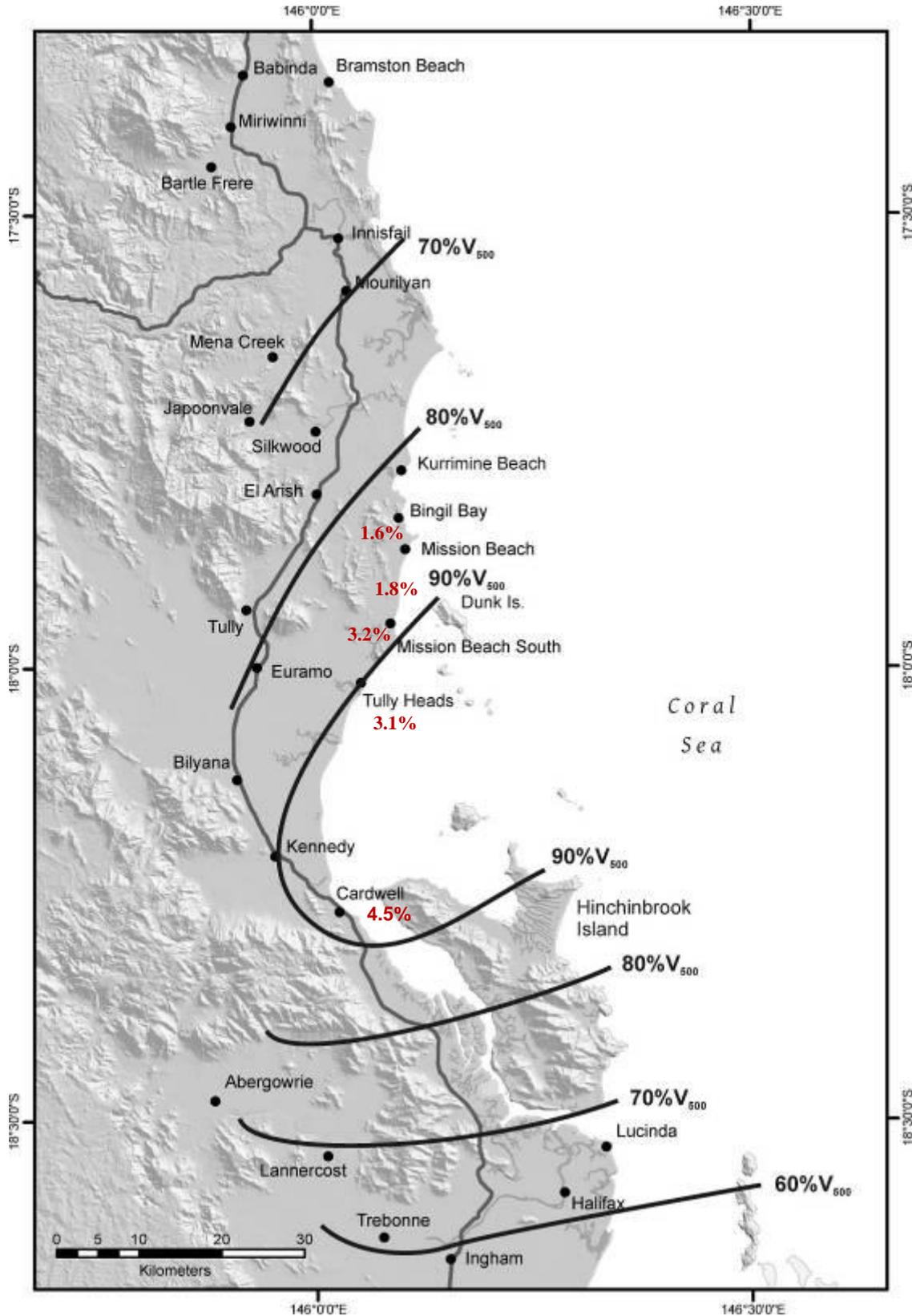
Figure 3.3 Estimated gust wind speed as a percentage of design speed for houses (Map also shows percentage of Post-80s houses in street surveys with roof DI >3)
