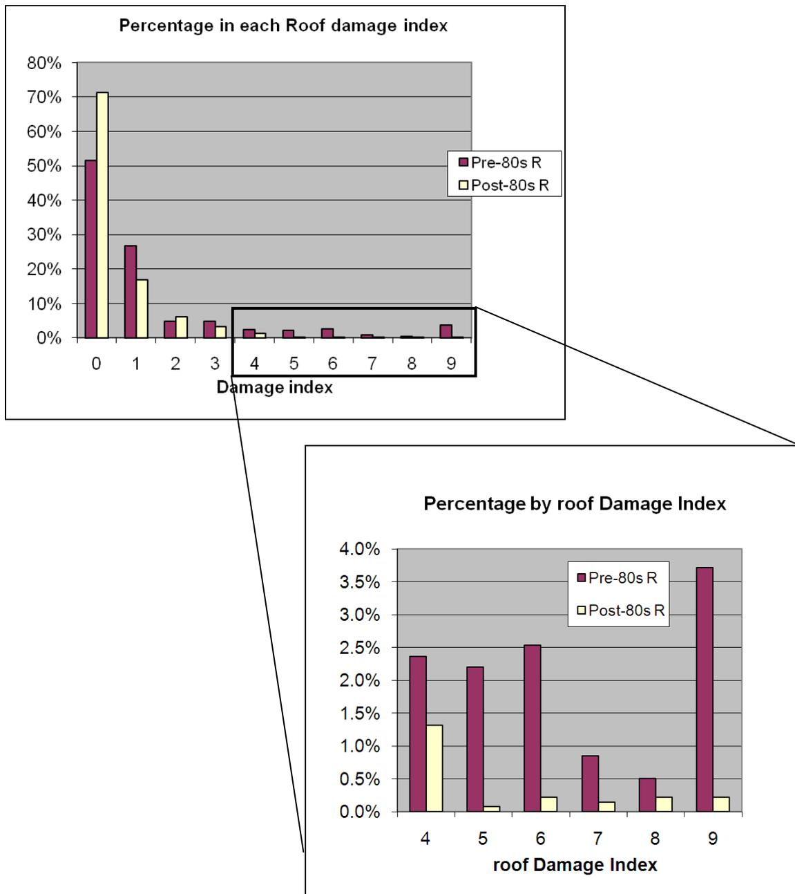
**Figure 3.2 Comparison of roof Damage Index by construction era across the study area (Refer Table 3.1 for Damage Index values)**
