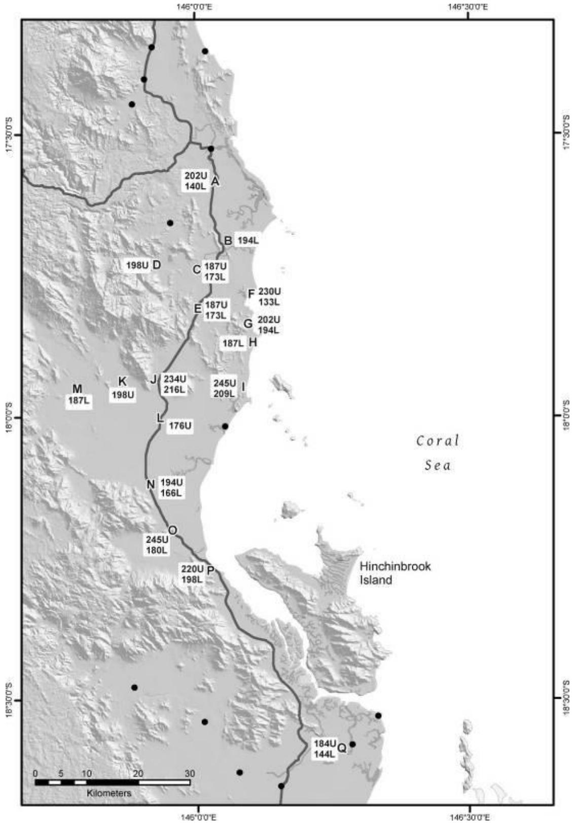
Figure 2.3 Upper and lower limits from “windicators” (km/h)
