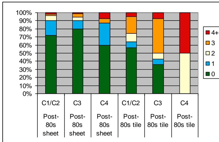
**Figure 3.31 Roof Damage Index for Post-80s houses
