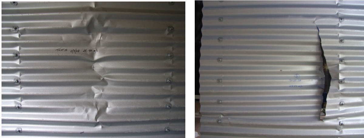
Figure 10: Corrugated wall cladding after impact at midspan (left) and close to internal support (right) by the 4 kg timber missile at 25 m/s
