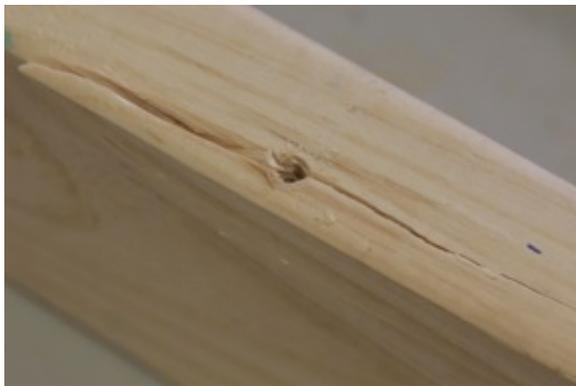
*Figure 3.6 Splitting of rafter with inadequate edge distance*
