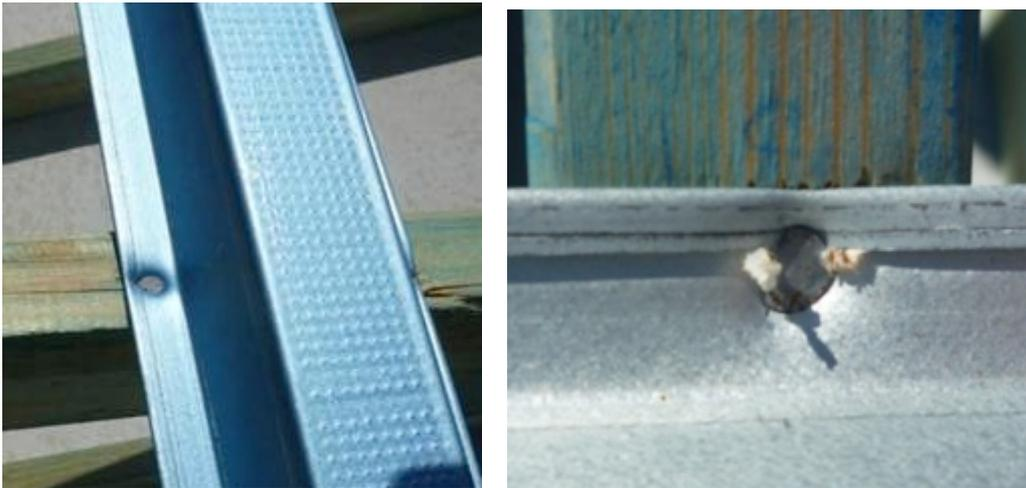
(a) deformed surface of batten      (b) punched through a batten
